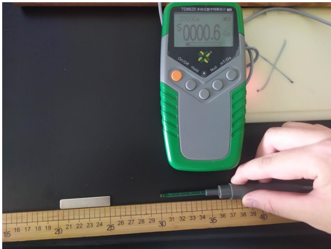
Figure 1. The magnetic field strength at 5cm far is almost zero
